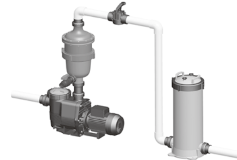
Installation with 2 way shut off valve
